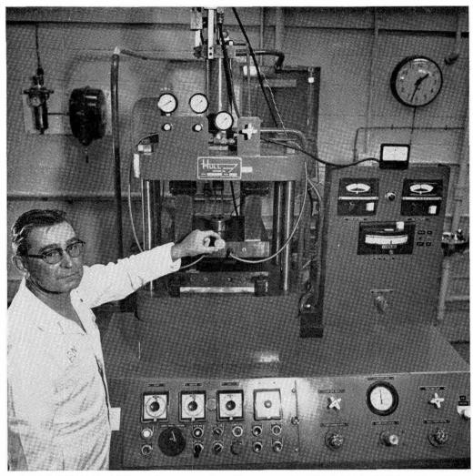
BEN LONGFELLOW (4222) displays pellet of epoxy material which is inserted into the transfer molding machine to encapsulate electronic components or to form small structural shapes. New machine enlarges capabilities of Sandia's Plastics Laboratory.
